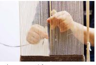
[Hand-woven carpets] Pile yarn is knotted in a figure eight one by one on the double warp yarn. This is the same method used in manufacturing Persian carpets. Being expensive, these carpets are often considered a form of artistic craft.
