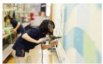
[Tango Hooked Rugs] These are called hooked rugs since U-shaped yarn loops are inserted, using equip- ment called a hook gun, into the base cloth set on a frame. Made with techniques originating from the traditional handwoven rug (Sakai-style rug) manufacturing, Tango Hooked Rugs feature a hand-woven texture, magnificence, and grandness.
