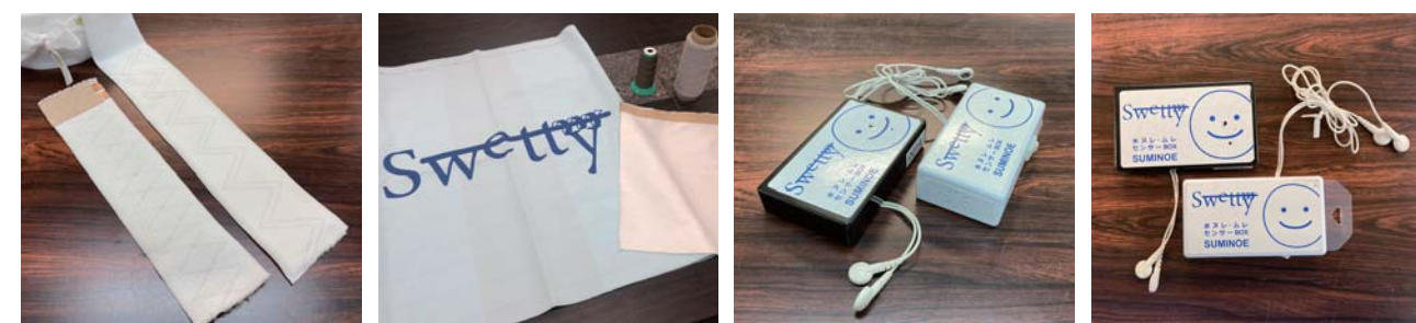
Water wetting detection fabric (in a ribbon shape)
